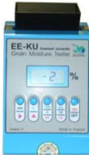
Put the grain on top of the opening. Press button
