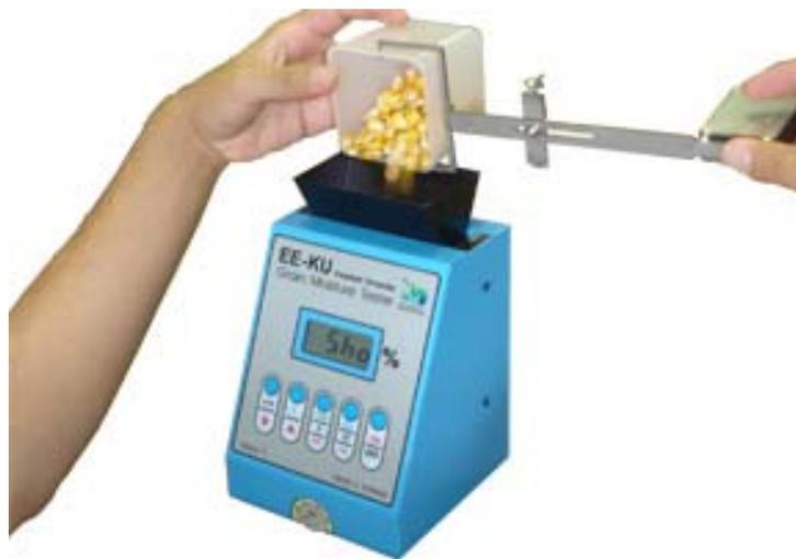
Note : pouring grains in to the opening slowly and gradually will give more accurate and less error of the measurement . But pouring the grains to fast will give little error with less percentage than the reality.
