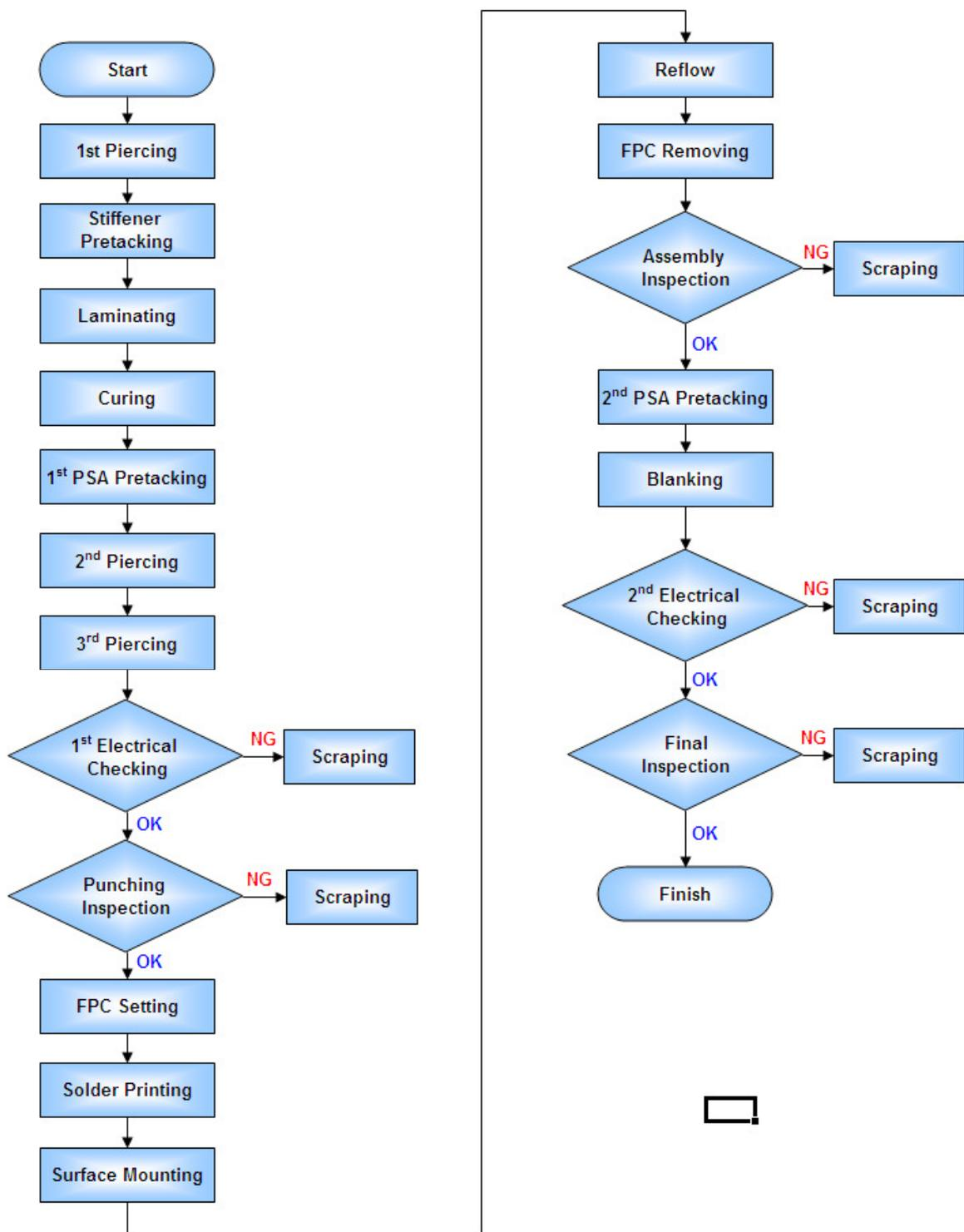
Figure 4: Process flow diagram.
