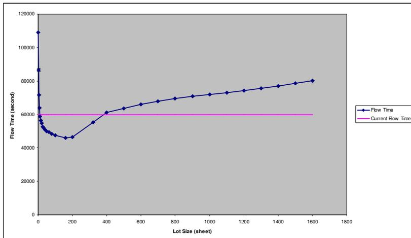
Figure 1: Flow time when the production lot sizes are varied.
