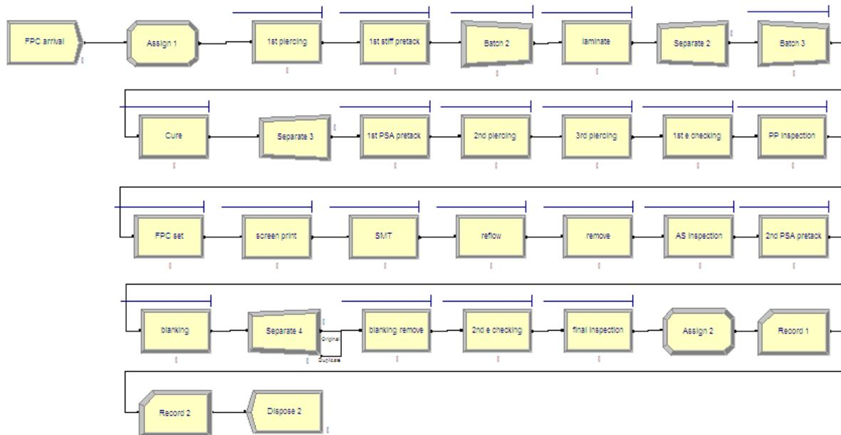
Figure 5: Simulation model of the current push system.
