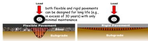
Figure 1: Rigid and Flexible Pavement Load Distribution
