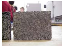
Figure 2.9: SMA Aggregate Structure. Notice the stone-on-stone contact of the larger aggregate particles.
