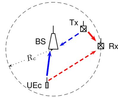
Fig. 1: The  $R_c$ -radius cell consists of D2D transmitter (Tx), D2D receiver (Rx), which is at the cell edge, the cellular user (UEc) whose uplink is shared with Tx, and the base station (BS). Assuming D2D mode is active, solid lines represent the desired signals while dashed lines represent the interfering signals.
