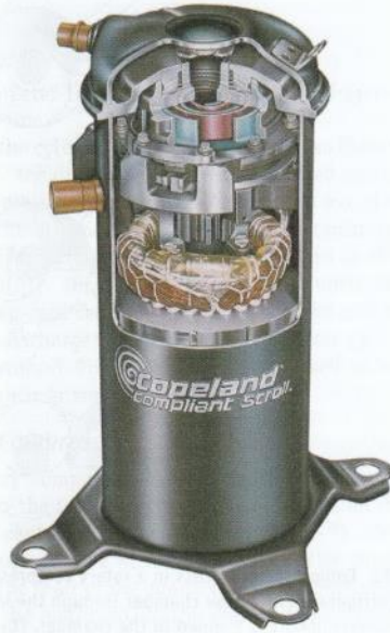
Figure 2-12 Scroll compressor. Courtesy of Copeland Corporation.
