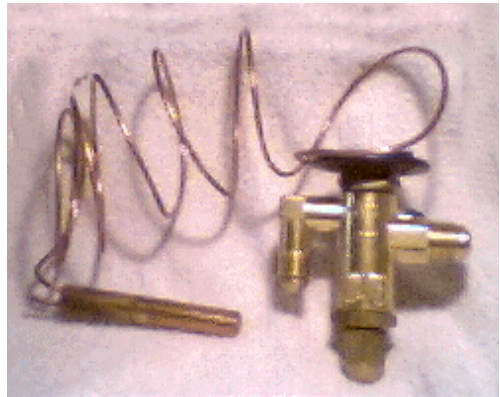
Mechanic expansion valve Thermostatic expansion valve (TXV)
