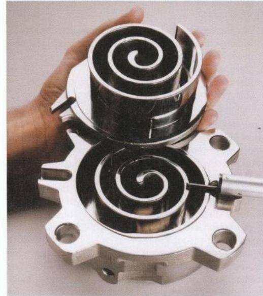
Figure 2-13 Two identical scrolls that form crescent-shaped pockets when nested together. Courtesy of Copeland Corporation.
